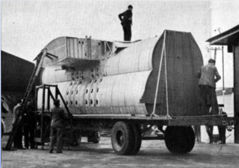
Half-scale fuselage section built for testing at Farnborough
