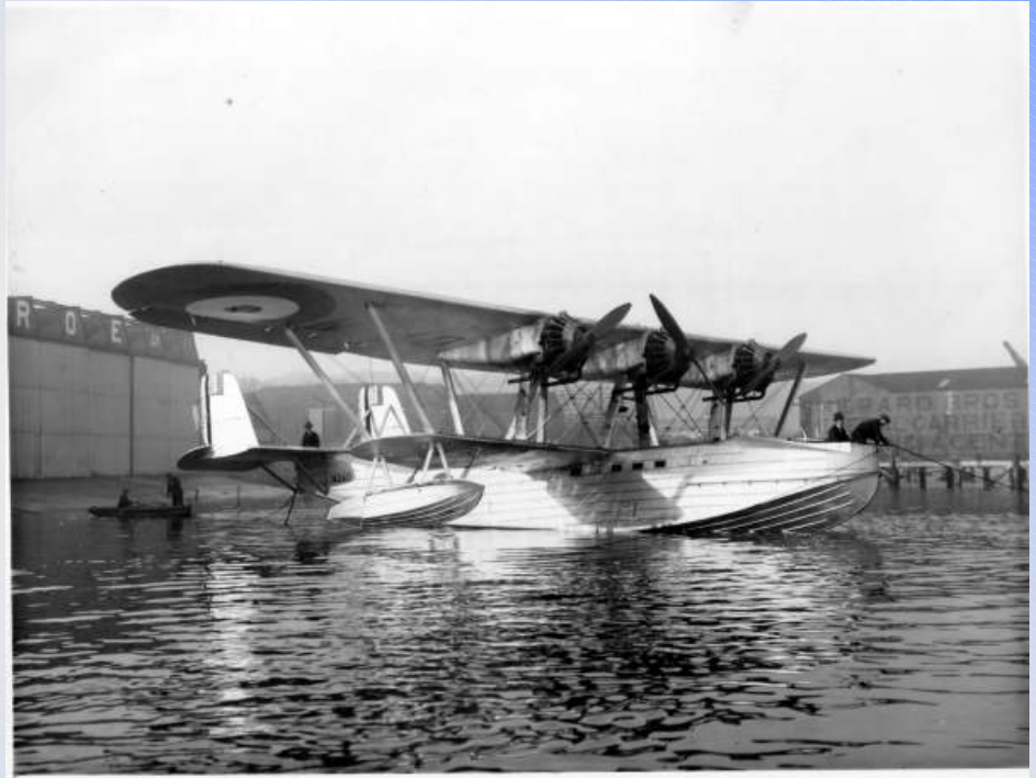
Saunders-Roe A7 Severn metal hulled flying boat moored off the Solent Works slipway at West Cowes c1930
