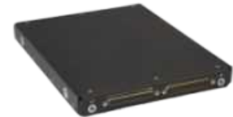
EFB computing unit – avionics bay
