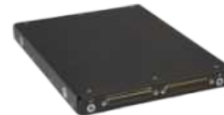
EFB computing unit – avionics bay
