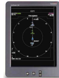
Goodrich SmartDisplay® Class 3 EFB displaying the ACSS SafeRoute™ Merger & Spacing (M&S) CDTI
