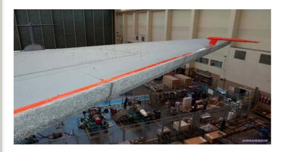
Handling Qualities remain outstanding despite the severe ice shapes in normal and failure conditions
