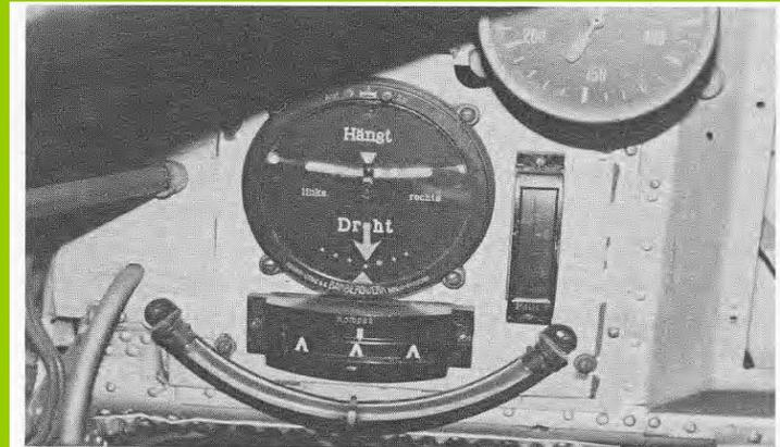
Captain Koehl's instrument panel showing the airspeed indicator (top) and the turn and bank (middle) with the remote compass indicator below. The climb/descent instrument is at the right and under everything is a large inclinometer. (F.W. Hotson)
