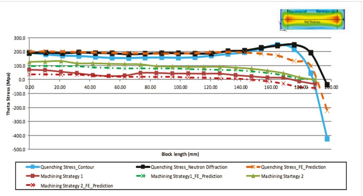
**Residual stress measurement and FE prediction after quenching and machining**
