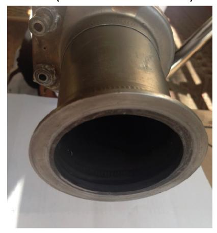
Visual inspection of a bleed air off-take port from a Boeing 737. The interior is black from oil contamination. (GCAQE 2017)
