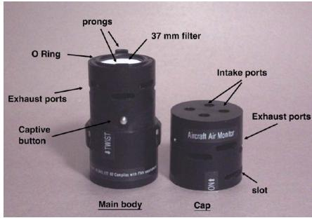
Prof. Van Netten invented this "VN-Sampler". It is not an in situ measurement device, but a means to collect the air in a fume event for later detailed analysis in a laboratory on the ground. The device is FAA approved.
