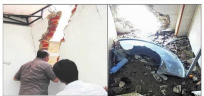
Figure 12: Property damage from a section of the No. 2 engine turbine disc
