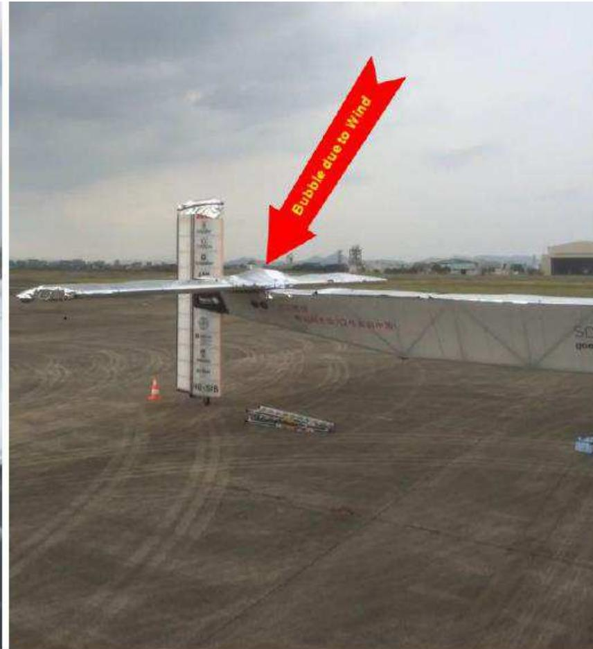
Fig deformed space blanket on the HSt
