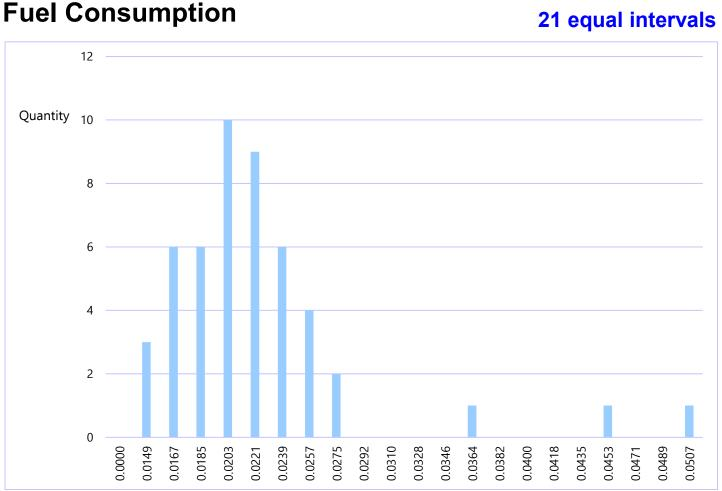
Normalized OEM-based fuel consumption per seat (kg/km)
