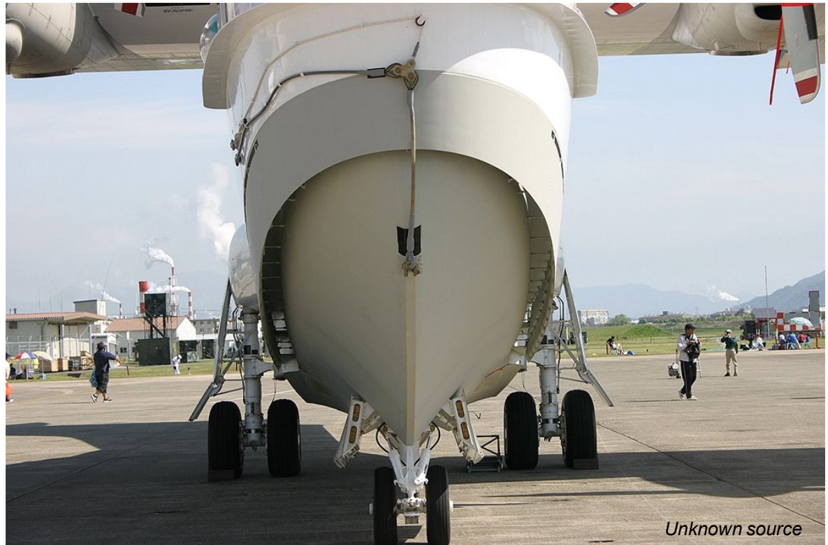
Bottom with Groove Type Spray Suppressor and fairing
