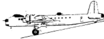
Tail wheel – type (retractable)
