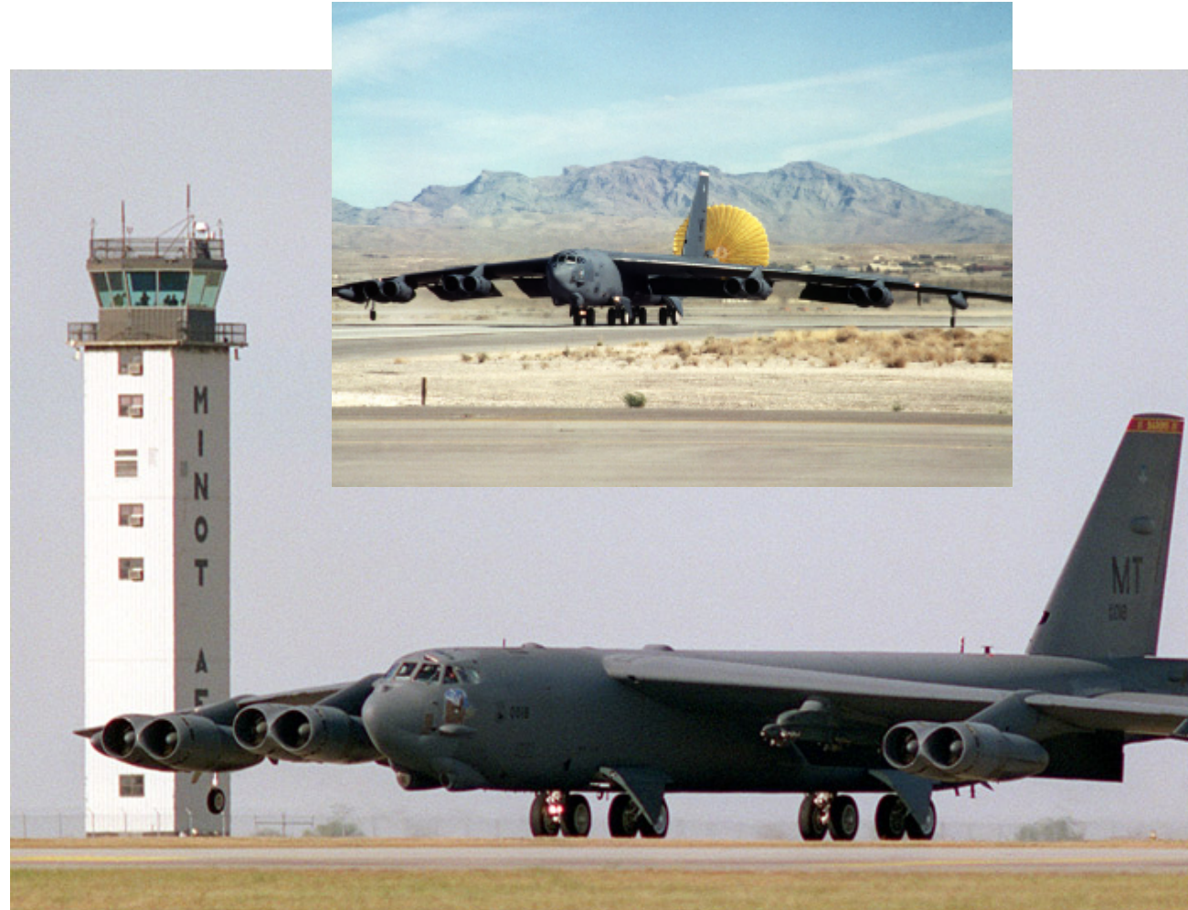
Tandem Gear , Boeing B-52 , 1954
