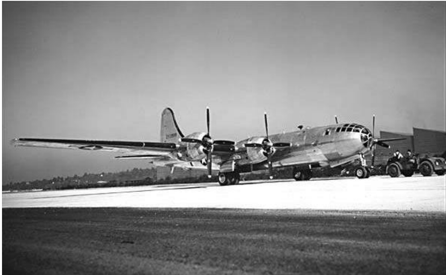
NLG-Type with Twin Wheels , B-29 , 1939
