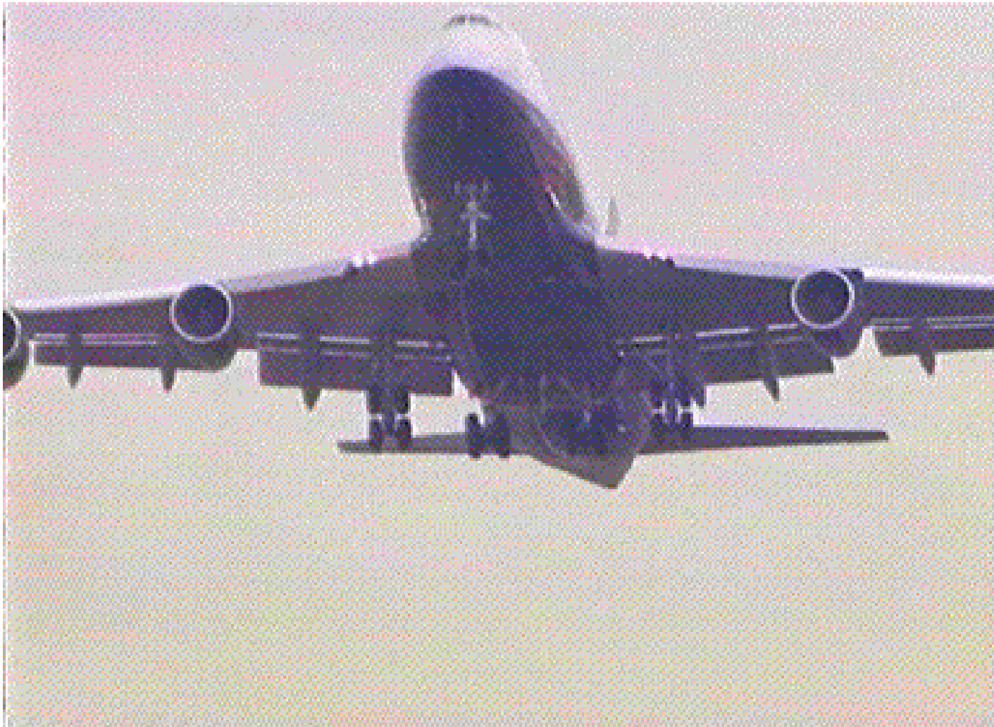
Landing Gear Retraction, Boeing 747
