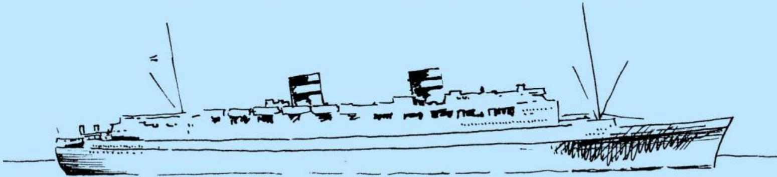
S.S. " Nieuw Amsterdam" 36982 tons, length 231 m., 21 kt. (1938) 556 1ST. CLASS, 455 2 ND CLASS, 209 3 RD CLASS.
