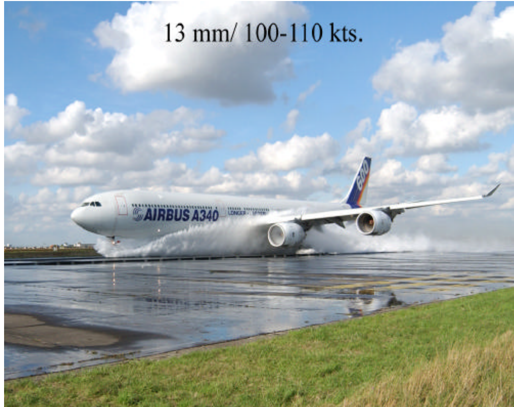
FLOODED RUNWAY SPRAY INGESTION FROM LANDING GEAR
